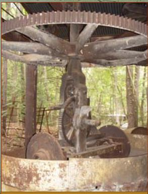
**Large Mill to Mix the Soils and Clays**
